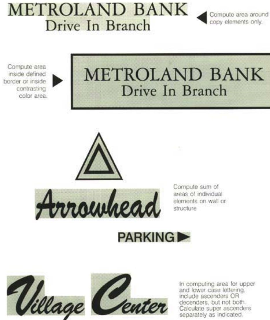
Figure 1003.4 SIGN AREA - COMPUTATION METHODOLOGY Sum of Shaded Areas Only Represent Sign Area for Code Compliance Purposes Signs consisting of individual letters, elements, or logos placed on building walls or structures
